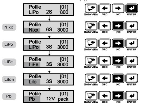
\* The programming setup is applied differently when you press START/STOP button less than 1 Sec and longer than 1 Sec
